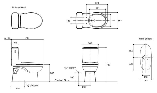
Note: The recommended dimension for installation can be adjusted according to user preferences and layout. Kohler Co. reserves the right to make changes in product characteristics, packaging, or availability at anytime without notice.
